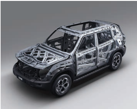
SAFE BODY STRUCTURE 85% HIGH-STRENGTH STEEL
